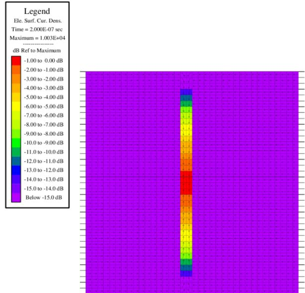
**Figure 3: Surface current density at early times in the simulation in Amperes/m<sup>2</sup>**
