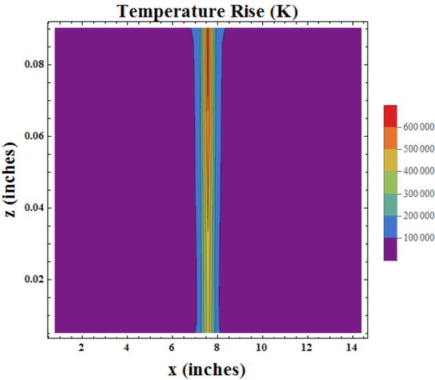
**Figure 6: Cross sectional view of the composite surface heating. The view is centered in the middle of the x axis.**
