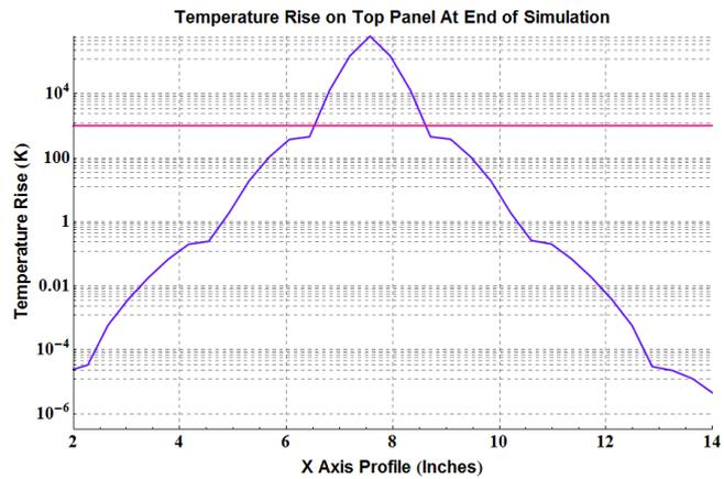
**Figure 5: Temperature profile along the x axis on the top panel at the end of simulation. The profile is in middle of the panel in the y-axis.**
