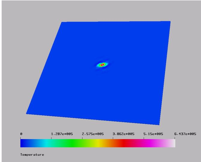
**Figure 4: 3D Elmer plot of the temperature profile of the CFC surface at the end of the lightning simulation. The heating is centered near the point of attachment.**
