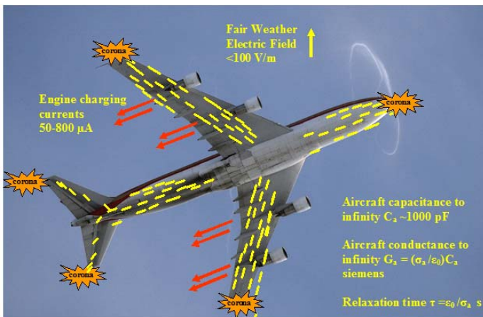
Aircraft electrostatic equivalent circuit
